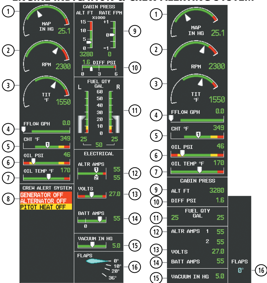
Mirage EICAS Display (Normal Mode)
